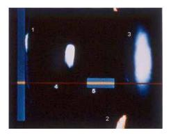
The instrument measures back-scattred light from small molecules such as proteins and this is called <u>laser flare photometry</u>. The measurement units of back scattered light from small molecules are <u>number of photons per miliseconds (ph/ms)</u>. The amount of back-scattered light is proportional to the concentration and size of proteins in the aqueous humor and is so indicating the level of inflammation.
